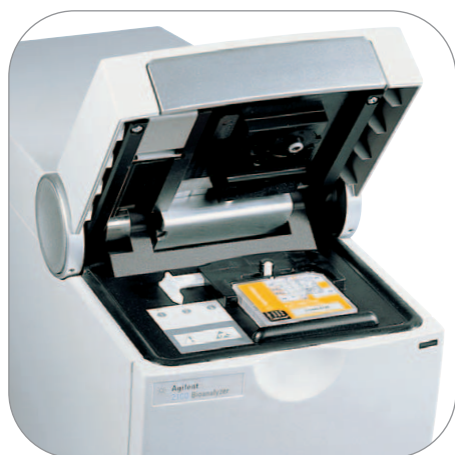
Agilent 2100 bioanalyzer with pressure cartridge and the cell chip included in the flow cytometry set.
