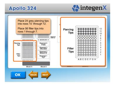
**NOTE:** Do not use the plastic carrier tray in Block 5, as it might cause tips to stick during automatic operation.
