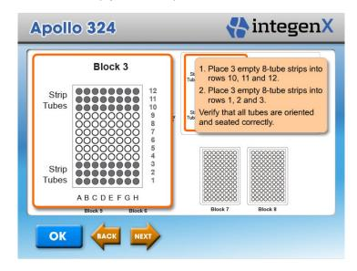
**NOTE:** Verify that all tubes are oriented and seated correctly.
