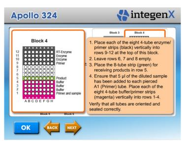
**NOTE:** Verify that all tubes are oriented and seated correctly.
